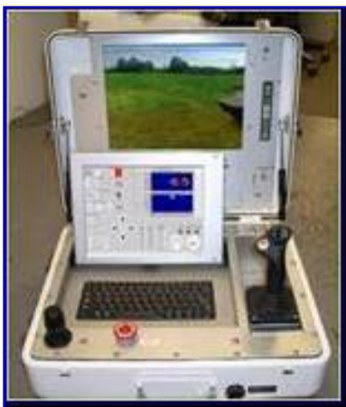
Figure 2. Operator Control Station (OCS)
