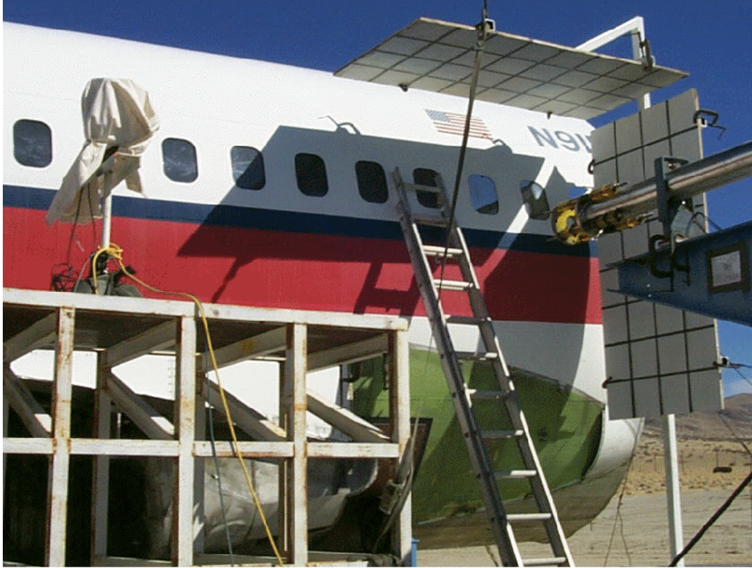
Figure 3. Test setup for full-scale evaluation of engine fragment barriers in the fuselage wall.
