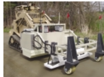
Figure 3. Nemesis robotic platform and detection sensor arrays
