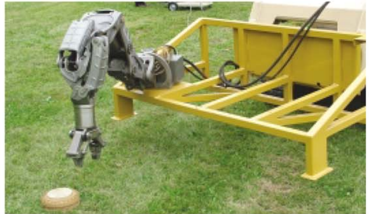
Figure 6. Manipulator arm with AT landmine
