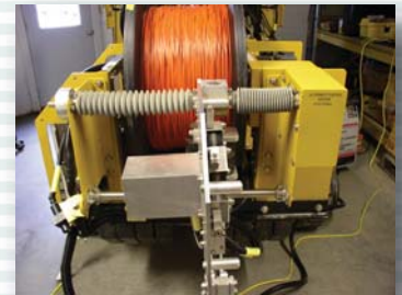
Traverse mechanism for even spooling
