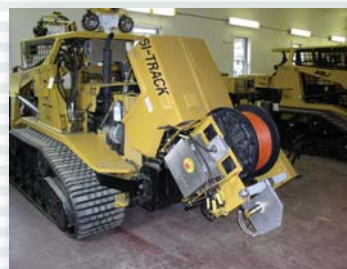
FCCS tilts with engine cover for easy access
