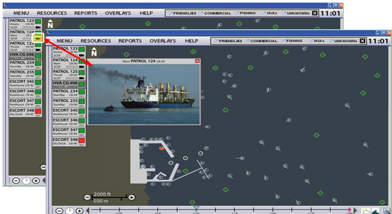
Figure 2. Camera icon in list of Patrol Boat information linked to camera on that patrol boat; reflects requirement for watch officers in the MOC to see the on-water view of patrol boats to aid in decision making.
